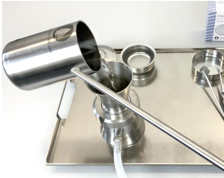
Figure 1 – Microbiological water analysis in remote places is easy and independent with the water sampler from LETZTEST.
