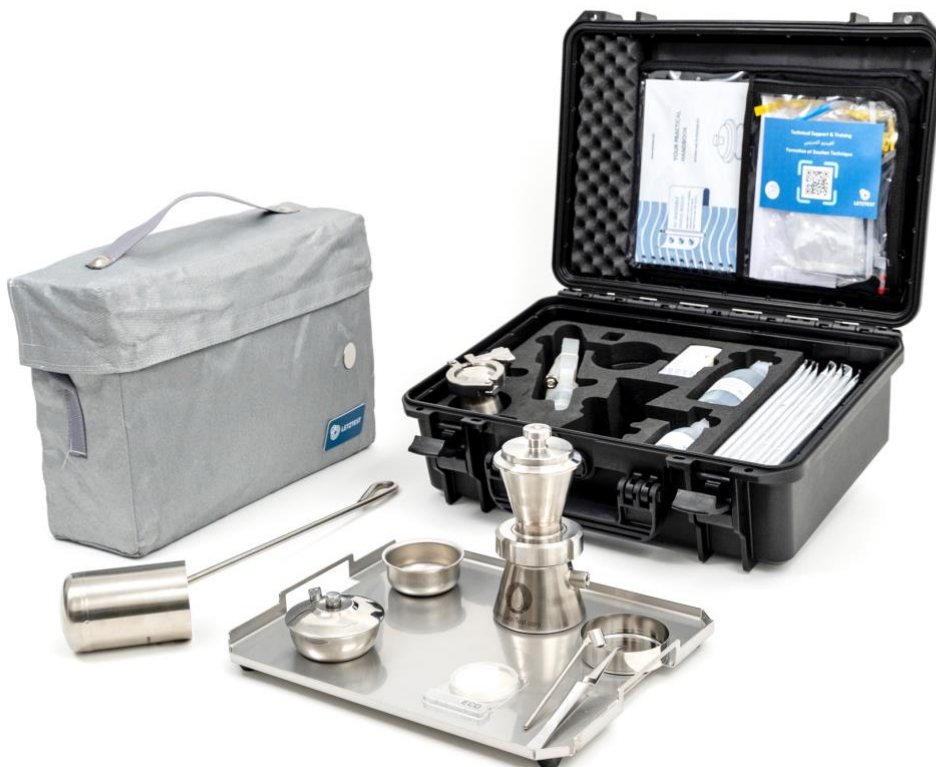
Figure 1 –LETZTEST Portable MIBI Water Lab - according to DIN EN ISO 9308-1
