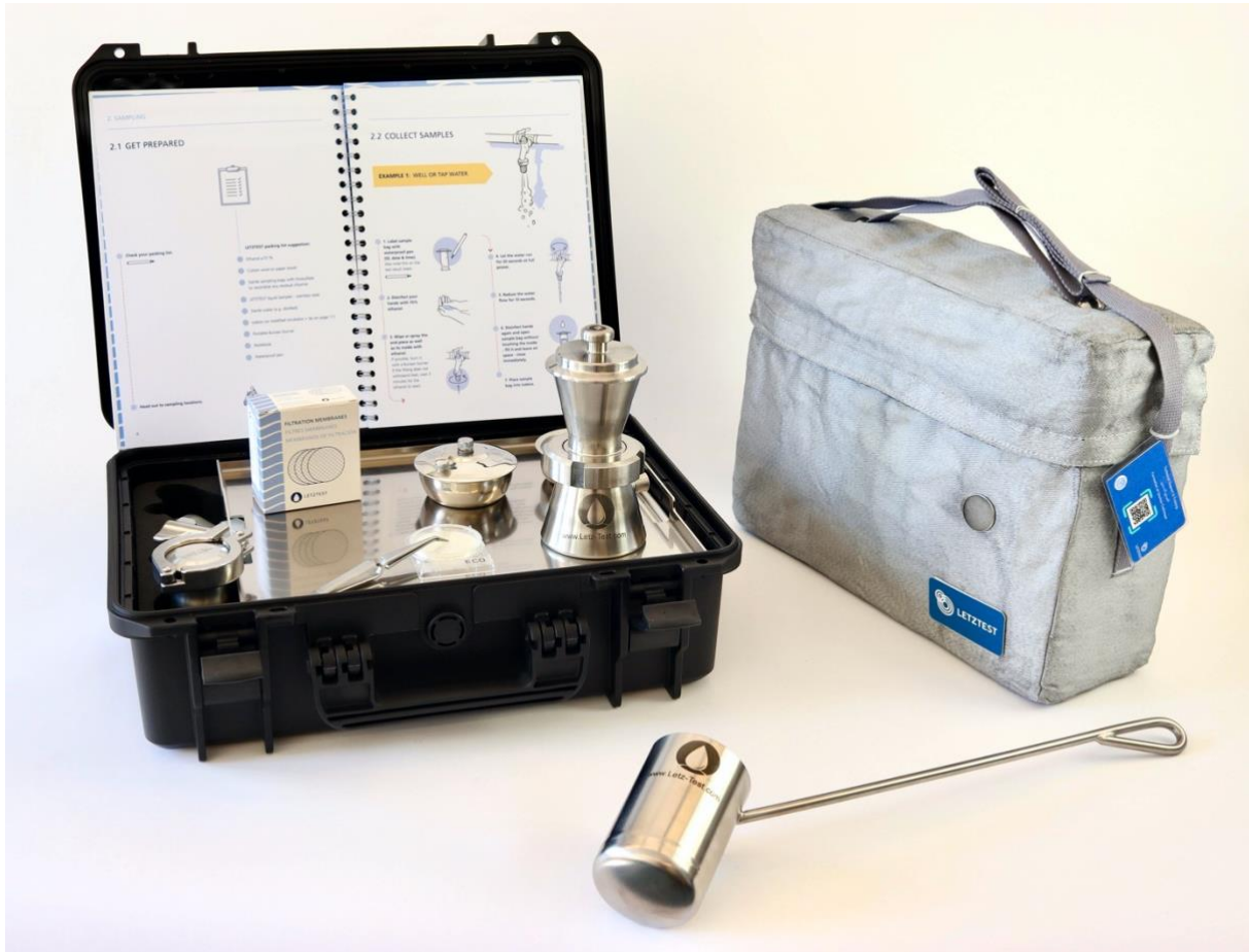
Figure 1 – The LETZTEST Portable Membrane Filtration Kit is part of the complete portable water microbiology laboratory by LETZTEST
