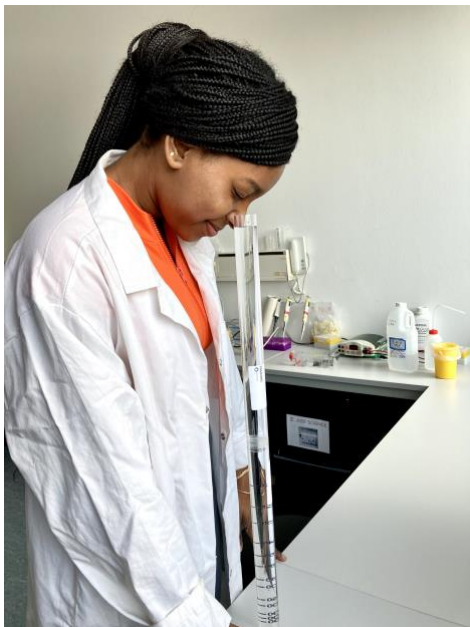
Figure 1 – The turbidity tube is a very user-friendly tool to measure the turbidity of water samples.
