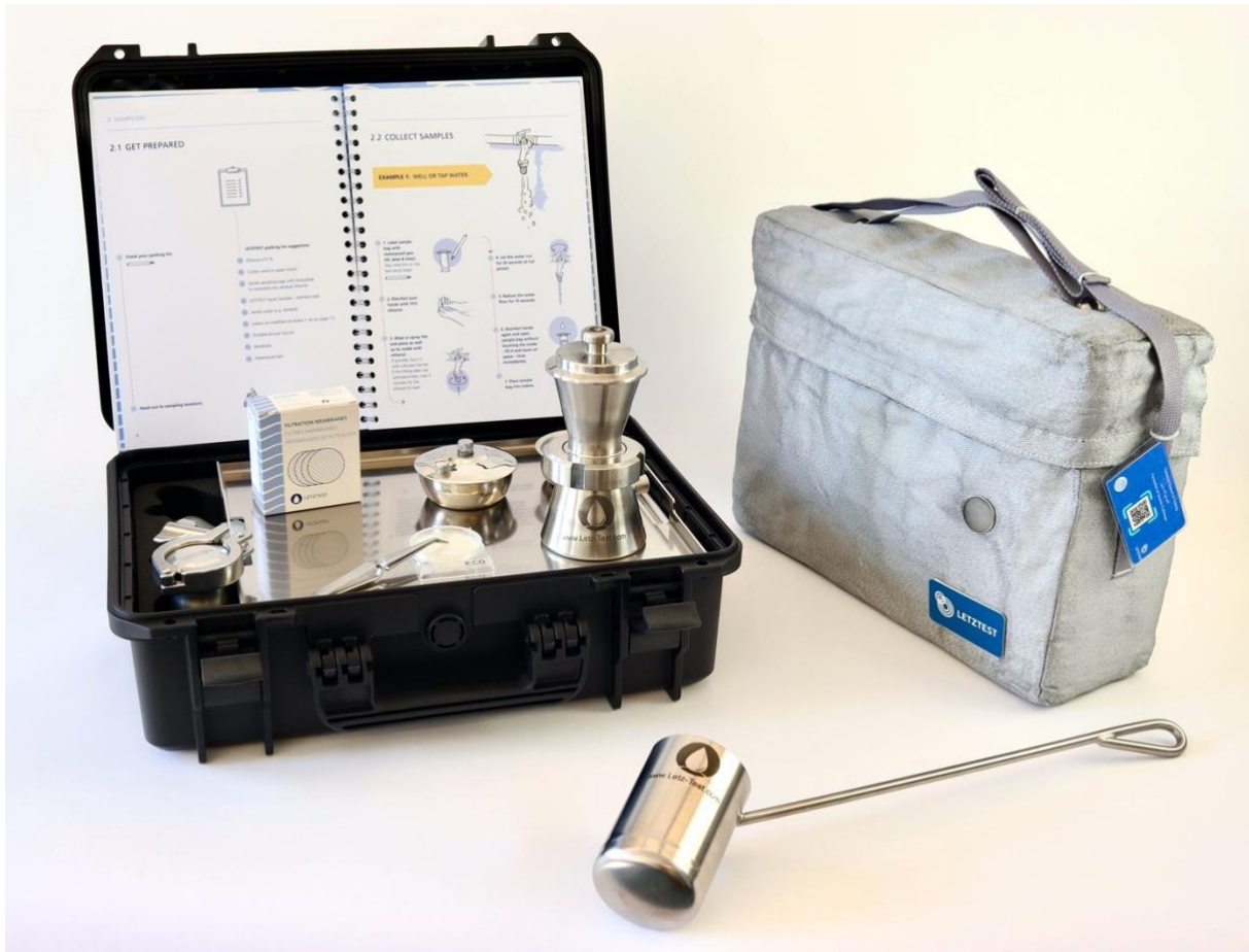
Figure 1 – The Portable Membrane Filtration Kit is part of the complete portable water microbiology laboratory by LETZTEST
